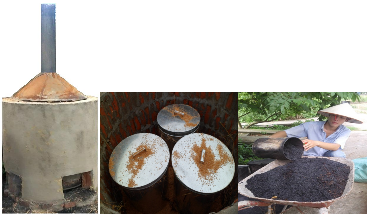
Figure 3: Production of Bio-char from inearobic charring of rice husk through indirect pyrolysis (fumigated husk)
